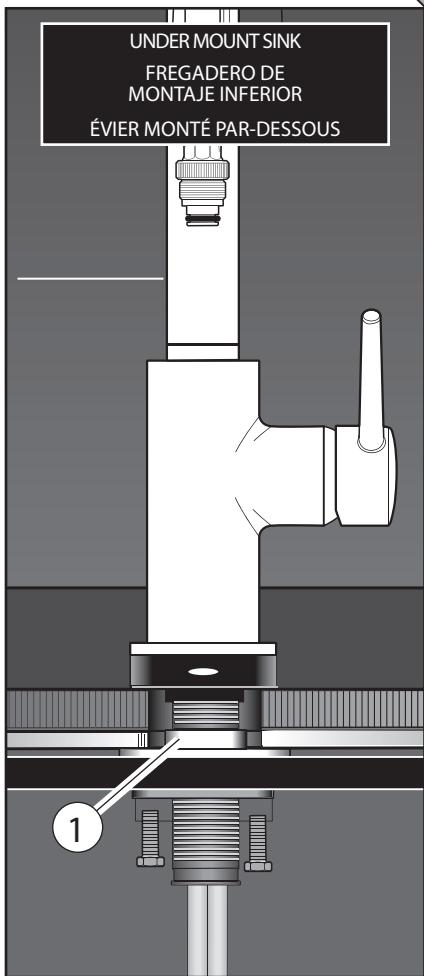
Lip (1) of isolation ring MUST fit into mounting hole.
