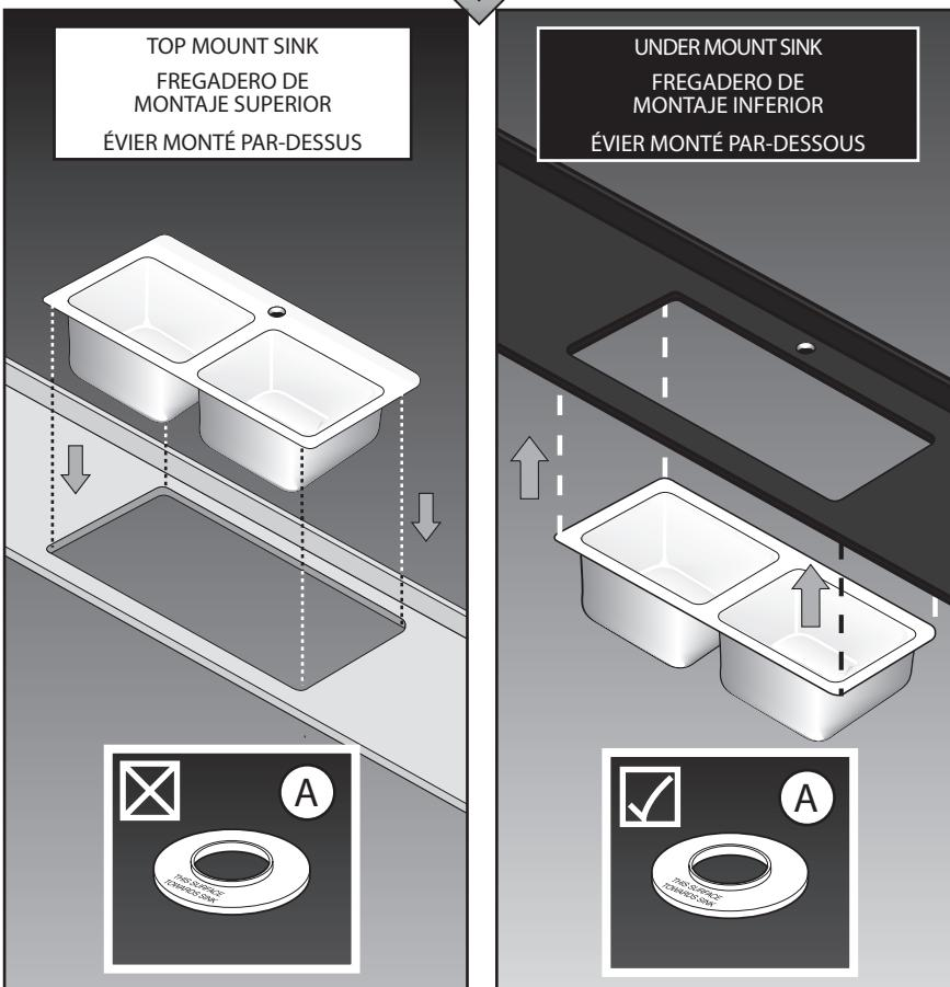
**TOP MOUNT** - If your sink is mounted on top of your counter as shown here, DO NOT use the under mount isolator (A) when installing your faucet.
