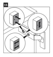
Back screw will adjust closer and further and front screw will adjust left and right.
