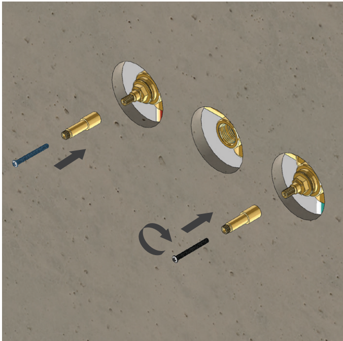
Insert stem extension on hot and cold handle and secure using provided screws
