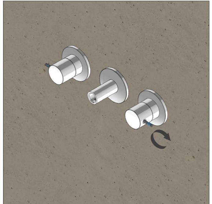
Tighten long hex screw to secure handle
