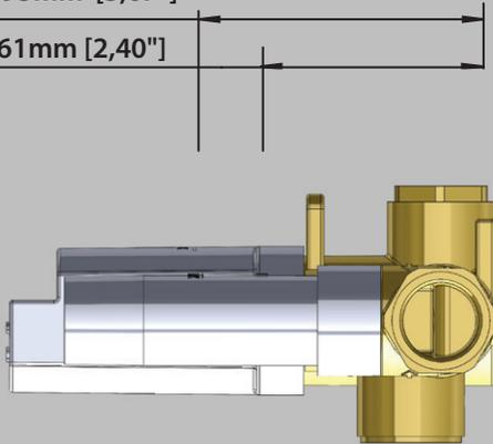
The distance between back of the valve to the finished tile surface should be between 2.40" and 3.67" inches.
