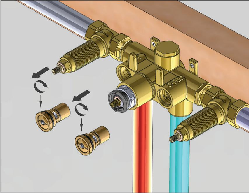
Use a spanner to twist in the shown position and remove supply stop
