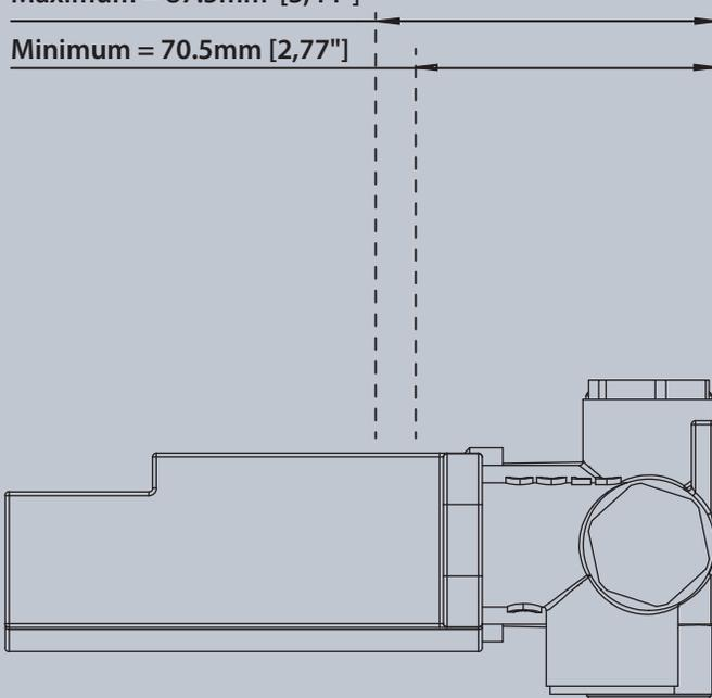
The distance between back of the valve to the finished tile surface should be between 2.77" and 3.44" inches.
