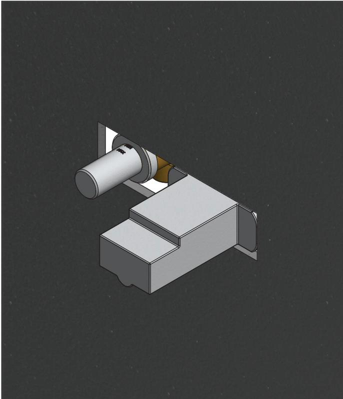
Install Drywall and Tile. Ensure finished tile surface is between the min and max marks on the mud guards.
