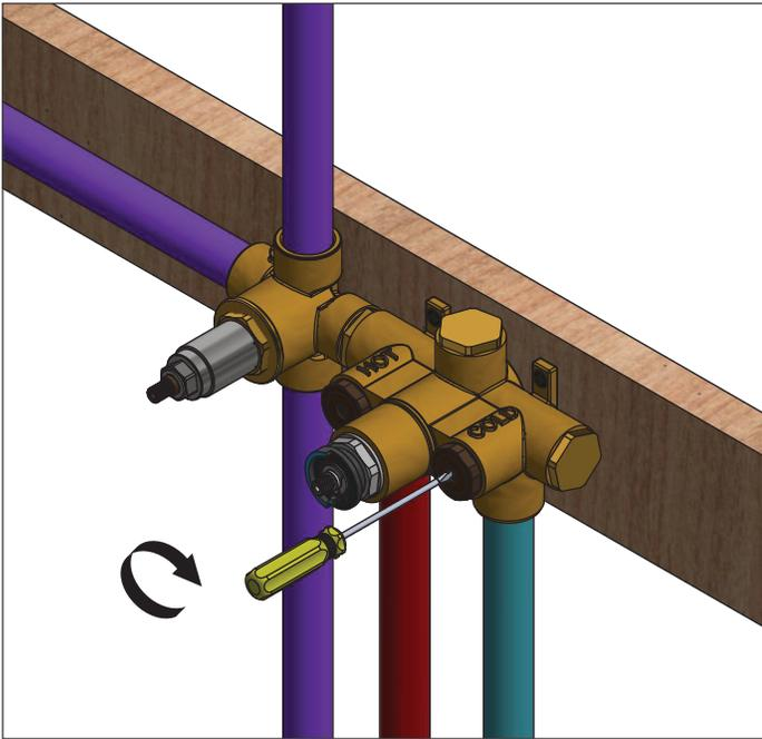
Turn Clock-wise 5 times to stop water flow.
