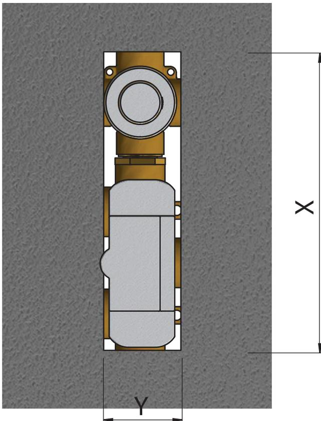
Isenberg's TVH Series valves comes with a black pre-attached mud-guard. This mud-guard is not to be removed or discarded. Its purpose is to guide the installation professional on the proper cut-out dimensions of the drywall.
