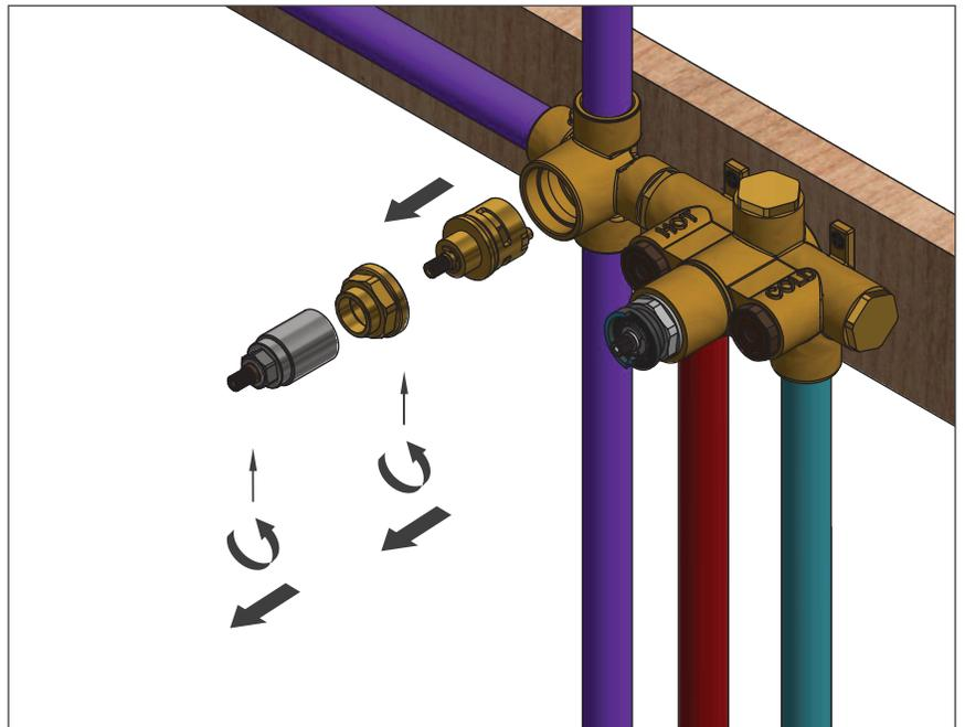
**INSTALLING EXTENSIONS TO THE VALVE - OPTIONAL - ACTUAL VALVE MAY VARY**
