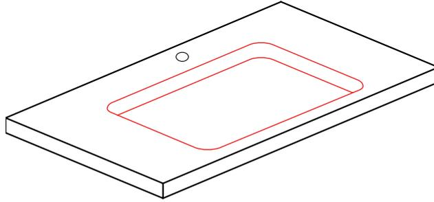
Measure the size of the sink. Cut the countertop to allow the sink slide in.
