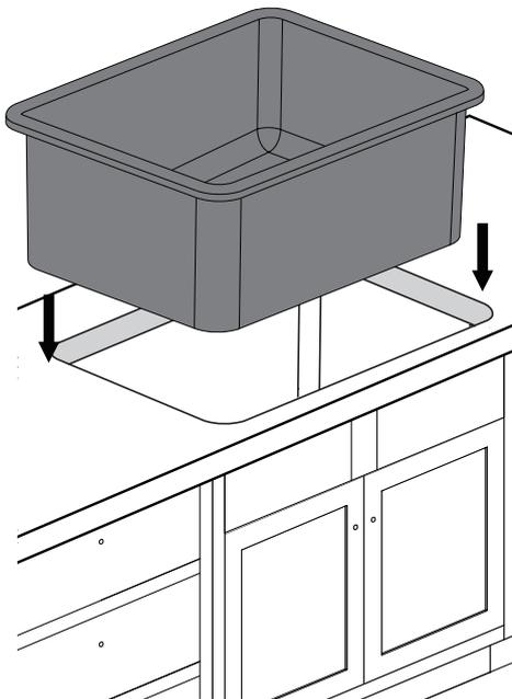
Insert the sink into the opening, check the alignment of the sink to the cutout in the countertop and press firmly.
