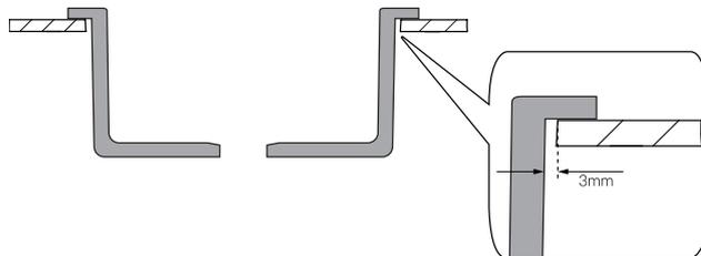
Subtract 3 mm from the width of the underside of the sink rim, and then subtract this amount from the perimeter you have drawn.
