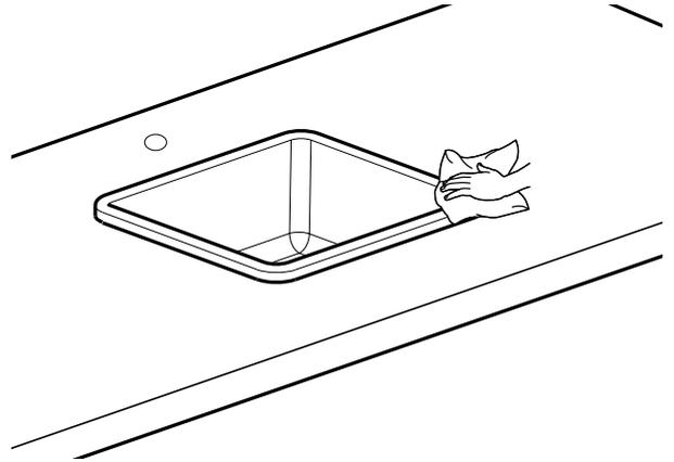
After cleaning, apply a bead of silicone sealant between the top flange (or lip) of the sink and the countertop to create a watertight seal. Clean excess silicone immediately. Verify the overall appearance and check for levelness to ensure correct drainage. Carefully place the countertop and verify that it is level.
