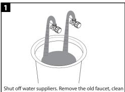
Shut off water suppliers. Remove the old faucet, clean the mounting surface.
