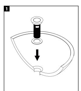
Remove all components from drain piece including: thin and thick silicone washer, hard washer, drain nut and tail piece.
