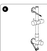
Mark the center slots of the upper mounting flange. Mark the center slots of the lower post and around the lower mounting post. Note: These are the points where you will drill holes for installing
