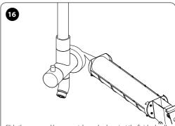
Slide the upper and lower escutcheons back against the finished wall. Apply silicone sealant to the rear lip of the upper and lower escutcheons.
