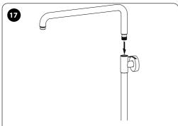
Assemble the overhead shower arm into the shower column. Ensure it is fully seated. Install 1 of the set screws into the shower column and tighten.
