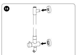
Assemble the upper escutcheon and lower escutcheon onto the upper and lower post of the shower column, respectively.
