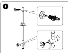
Hand tighten upper mounting flange onto inlet fitting. Insert the lower mounting post into the lower post of the shower column, tighten hex screw with hex wrench supplied. **Note:** Shut off water suppliers.
