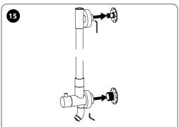
Install the shower column onto the inlet fitting and lower mounting post. Then use the hexagonal wrench to tighten the hexagon socket screw set.
