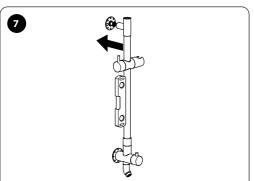
Install the shower column onto the inlet fitting, ensure there is no gap between the shower column and the inlet adapter. Lever the shower column.
