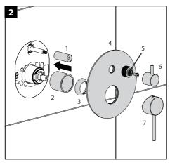
Remove two round mud guards by turning counter-closewise and discard. Remove the rough-in box and discard.
