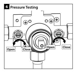
With both check stops in the fully OPEN position, turn on cold and hot water supplies and conduct a system water pressure leak test.
