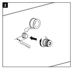
Wrap plumber's tape around the threaded ends of the 1/2" (13 mm) pipe nipple (not provided), then proceed to attach the Quick Connect onto the pipe nipple's threaded end.
