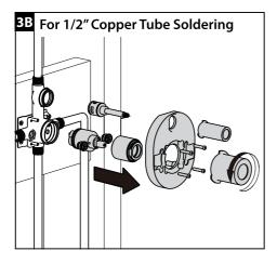
Solder water supply tube to the valve body. Note: Prior to soldering remove check stops, pressure balancing cartridge and diverter cartridge. Remove check stops by loosening hex nut counterclockwise. Remove the pressure balancing cartridge and diverter cartridge by unscrewing retaining nut with an adjustable wrench. Avoid soldering excessively at high temperature.
