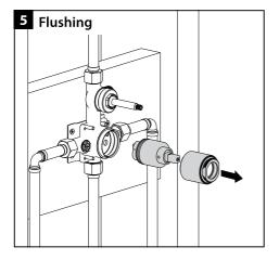
Remove pressure balancing cartridge by unscrewing retaining nut with an adjustable wrench.
