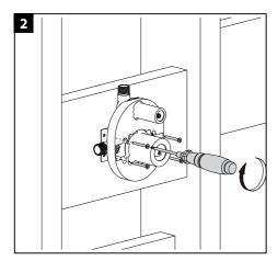
Install the body so the surface of the finished wall is flush with the front of the rough-in box. Make sure the word "UP" are on top of the valve body when installing.
