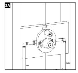
Connect the valve body to water supplies using proper fittings (copper tubing, iron pipe or PEX). **Note: For PEX, be sure to use the right fitting for crimping and the right tool for cold expansion.**
