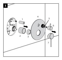
Remove cartridge handle(7), diverter handle(6) and Gear Cipher Adapter(5). Remove the trim panel(4). Remove the decorative ring(1) and decorative sleeve tube(2).
