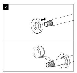
Slide escutcheon over shower arm, and apply Teflon tape onto male threads.
