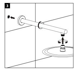
Screw the shower arm into threaded adapter. Screw the shower head onto the shower arm and tighten with an adjustable wrench.
