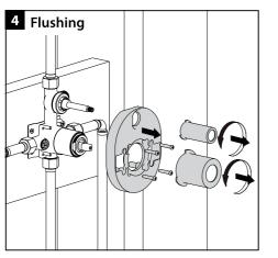
Remove two round mudguards by turning counterclosewise. Remove the rough-in box.
