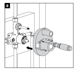
Reinstall rough-in box , two round mudguards by turning clockwise and complete the wall finish installation.
