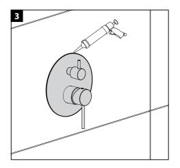
When firmly securing the trim plate onto the wall, apply a thin layer of silicone sealant around its perimeter to prevent water splashes from entering the wall.
