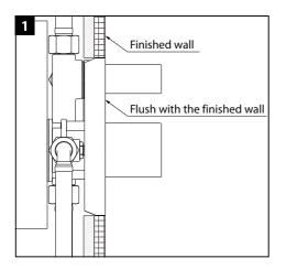
SHUT OFF WATER SUPPLIES. Consider the type and thickness of your finished wall before placing your stringer back plate.
