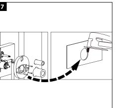
Use the rough-in box as a template to cut the wall properly.
