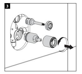
Remove the retaining nut using an adjustable wrench.
