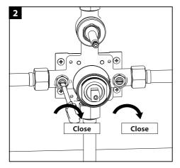
Using light force only, turn 2 check stops clockwise to close the check stops with the flat head screwdriver, until you feel resistance, the check stops are in the closed position.
