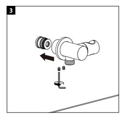
Place the escutcheon over the hand shower holder, then attach the hand shower holder to the quick connect. Secure it in place using the provided Allen key.
